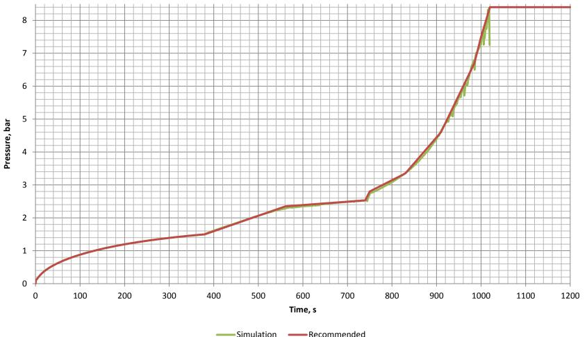
Recommended pressure-time dependence curve is also given, smoothed and supplemented with a constant pressure final calibration stage
