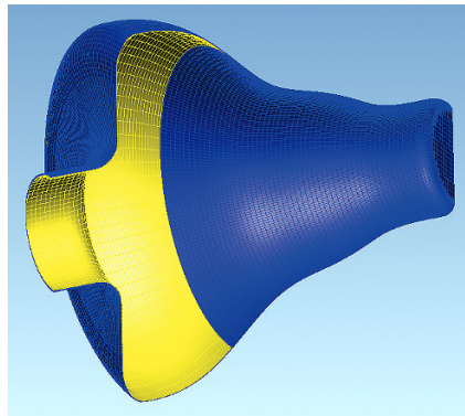
Fig. 13. Results from modeling the process of forming with a sliding edge over a fixture with an integrally concave surface.
